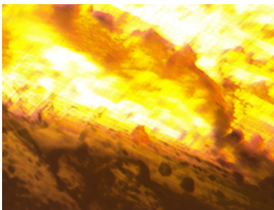
Gambar 20. Struktur Mikro Ferrite-Pearlite Baja S45C
